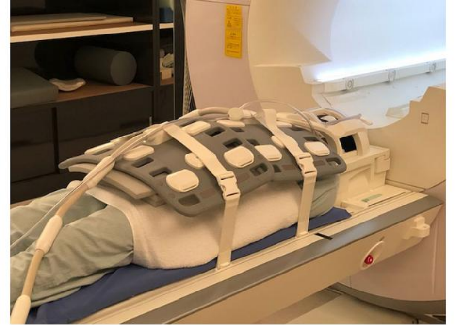
Fig. 5 Multichannel coil: 20-channel head coil, 32-channel spine coil, and two or three 18-channel body-array coils were combined to cover the area of Batson’s venous plexus, which is an area with a predilection for bone metastases
